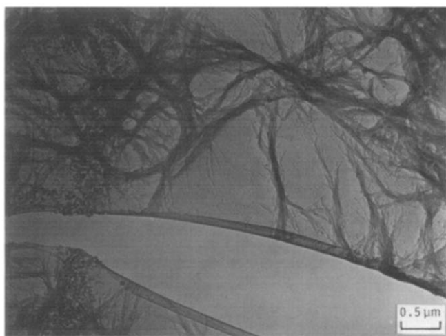
Figure 8 Transmission electron micrograph of BTDA 3, 3'-DDS dried in moist air after holding in a 1% solution in dimethylacetamide for 24 d. (Pt-Pd shadowed)
